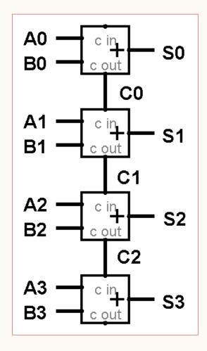
Now we've gone from adding 2 bits (A, B) to adding 3 bits (A, B, C\_in), we can look at connecting these building blocks to add numbers with more than one bit each!
