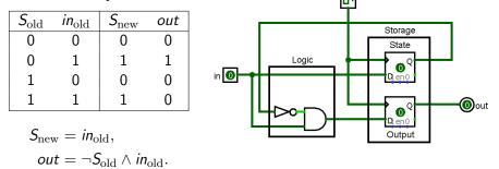
Much better! Notice we could also remove the NOT gate if we wanted, by using the Q' output of the state flip-flop instead of the Q output.
