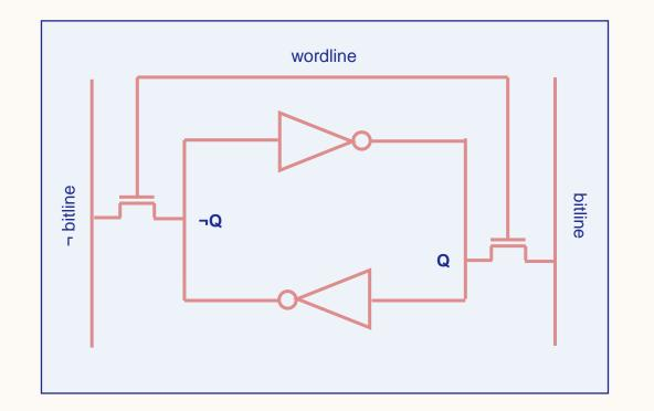
It's the presence of these **cross-coupled inverters**, that creates a bistable circuit and stores the bit value, as if Q = 0, then  $\neg Q = 1$ , then Q = 0 etc...
