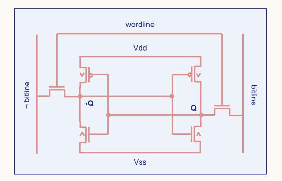
A SRAM cell has two outputs; *bitline* and ¬*bitline*. When the *wordline* input is high, both n-type transistors it's connected to are turned ON, which allows a data value to be transferred to or from the bitlines.
