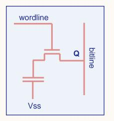
Turning the transistor ON (to read or write to the DRAM cell) will make the capacitor discharge a little. Even when off, the transistor leaks current, hence the need to **refresh periodically**, even if we don't access a cell.
