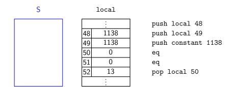
Logical comparisons work the same way. For example, the eq command pops the top two values of the stack, checks whether they're equal, then pushes the result back onto the stack.
