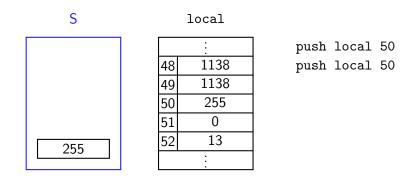
All arithmetic operations in Hack VM happen via the stack. For example, to add two numbers, we use the add command (which has no arguments).
