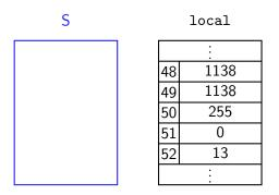
All arithmetic operations in Hack VM happen via the stack. For example, to add two numbers, we use the add command (which has no arguments).
