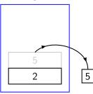
The Hack VM is an example of a **stack machine**, in which a stack takes the place of registers for arithmetic/logical operations and memory is used only for storage.
