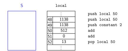
All arithmetic operations in Hack VM happen via the stack. For example, to add two numbers, we use the add command (which has no arguments).
