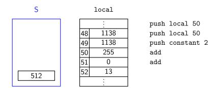
All arithmetic operations in Hack VM happen via the stack. For example, to add two numbers, we use the add command (which has no arguments).
