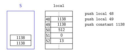
Logical comparisons work the same way. For example, the eq command pops the top two values of the stack, checks whether they're equal, then pushes the result back onto the stack.
