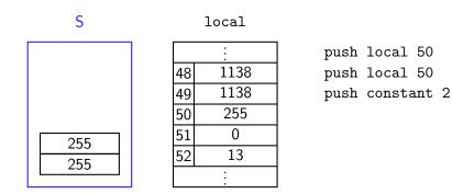
All arithmetic operations in Hack VM happen via the stack. For example, to add two numbers, we use the add command (which has no arguments).
